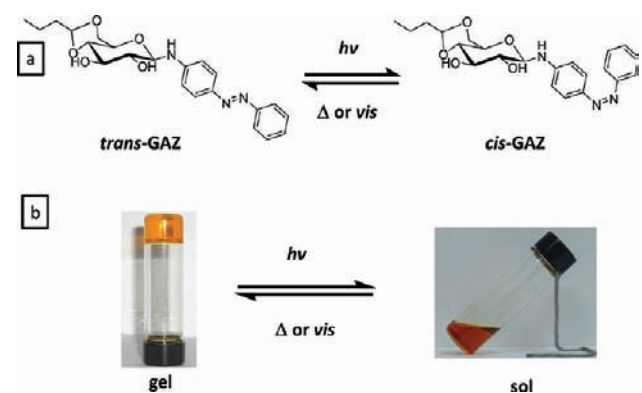
Figure 1. (a) Photoisomerization of trans -GAZ to cis -GAZ. (b) Gel–sol transition photograph of GAZ in toluene ( 1 \times 10^{-3} M).
